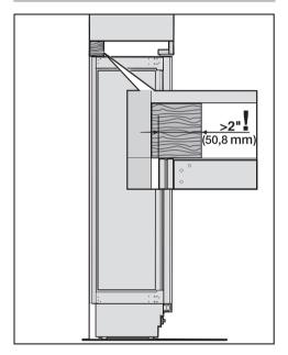
Cut a wooden beam (cross section min. 3" x 4" [75 cm x 100 cm]) to the required length.
